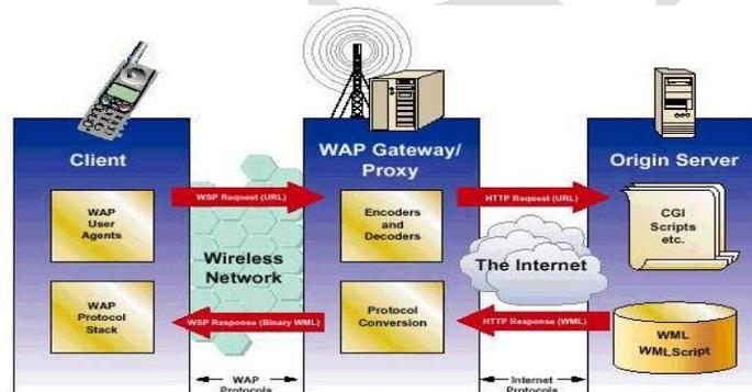
The *deck of cards* metaphor is designed specifically to take advantage of small display areas on handheld devices. Instead of continually requesting and retrieving cards (the WAP equivalent of HTML pages), each client request results in the retrieval of a deck of one or more cards. The client device can employ logic via embedded WMLScript (the WAP equivalent of client-side JavaScript) for intelligently processing these cards and the resultant user inputs.
