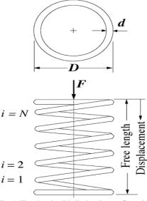
Fig. 1. The closed coil helical spring configuration
