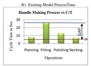
In the above processes the maximum cycle time is occurred in the fitting operation. In order to balance the cycle time of fitting operation in the handle making process, Polishing operation cycle time 13 seconds is considered as a line for balancing other operations. This is achieved through step by step modification in the cellular layout of the process.
