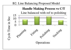
In the manufacturing process line it is balanced according to the cycle time of Polishing operation which greatly depends on the Number of operators, Number of machines, Available Space, Inventory, Operator Movement and cost. In this approach line balancing is achieved through modifying the current process layout.
