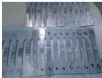
Figure 5: TS Welded samples cut by EDM
