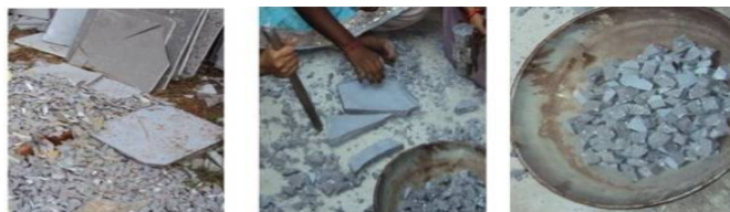
Fig 2. Shabath waste source manual cutting and preparation of aggregate
