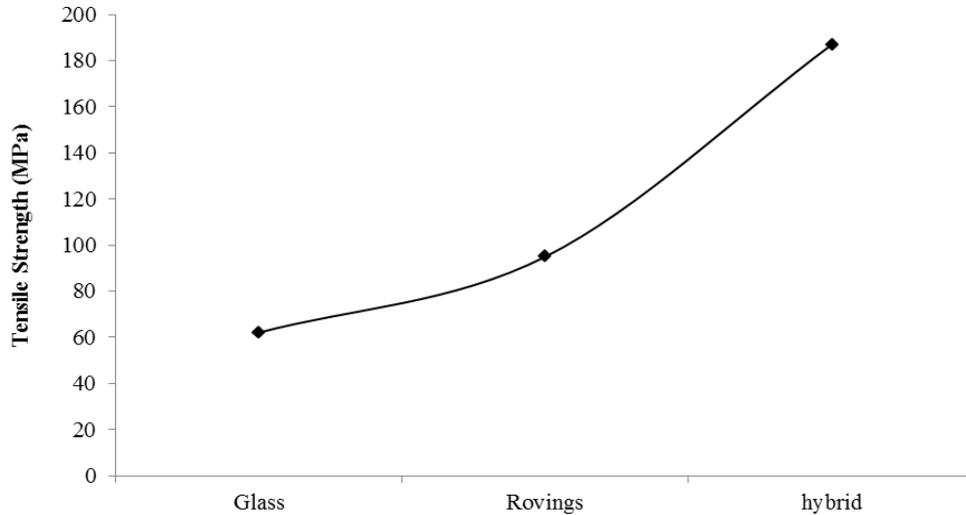
Figure 5: Ultimate tensile strength values of various fibers
