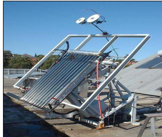
**Figure : Indoor experimental setup: Tube heat measurement**
