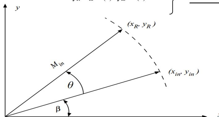
Figure 4:- Rotating the input vector by  $\theta$
