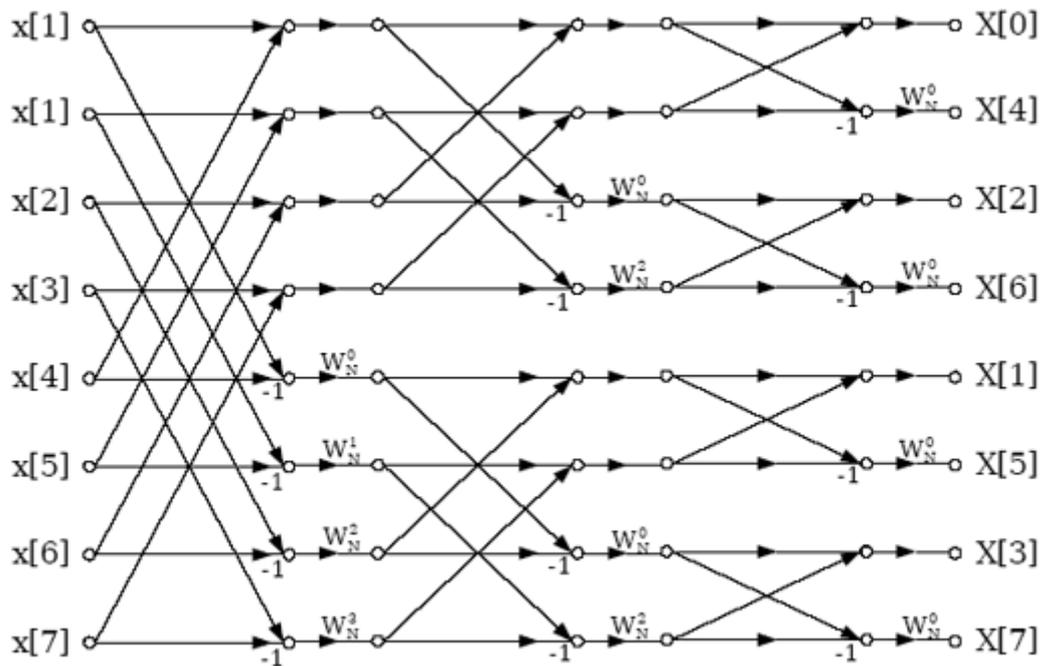
Figure 2: Radix-2 decimation-in-frequency FFT for a length-8 signal
