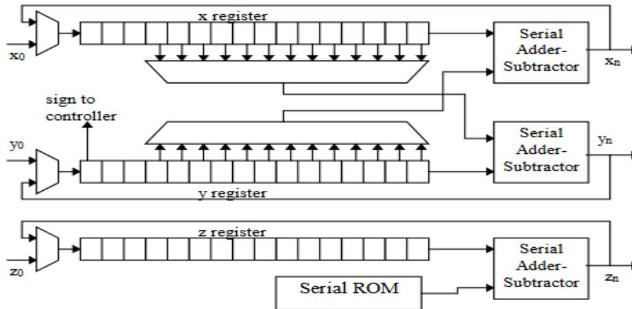
Figure 7:- Bit serial iterative CORDIC
