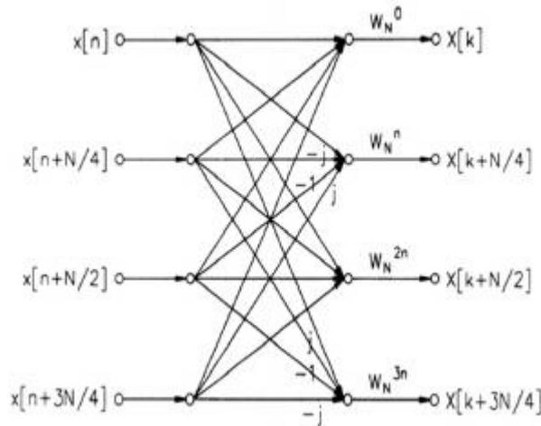
Figure 3: Radix-4 FFT Algorithm
