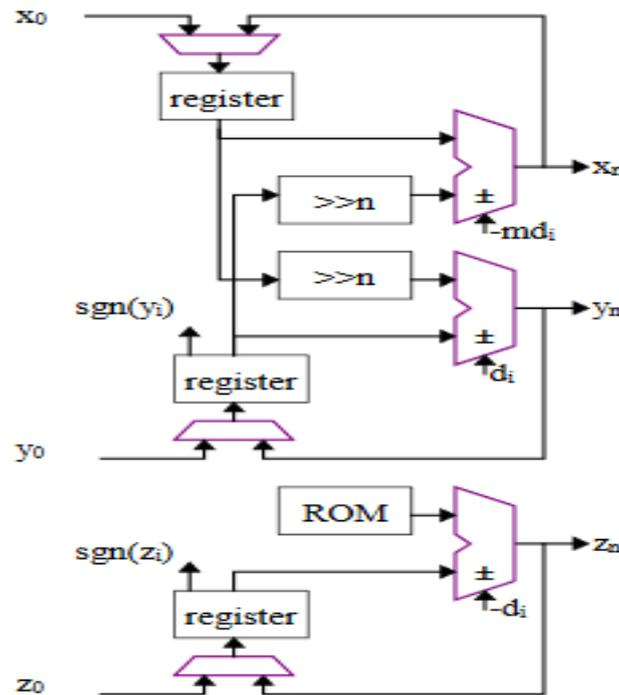
Figure 6:- Iterative CORDIC structure
