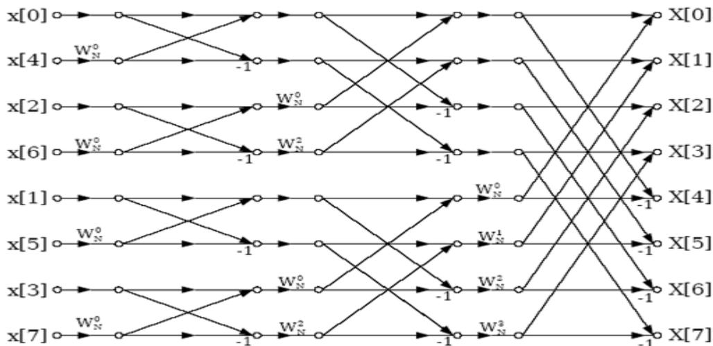
Figure 1: Radix-2 Decimation-in-Time FFT algorithm for a length-8 signal
