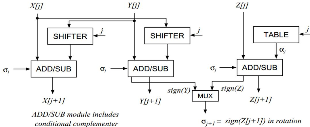
Figure 5. Implementation of Equation 4 for one iteration
