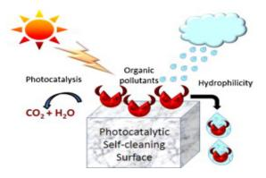
Figure 4: Self-cleaning activation process by UV light
