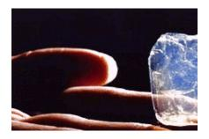
Figure 9: Aerogel insulation the lightest solid material on earth
