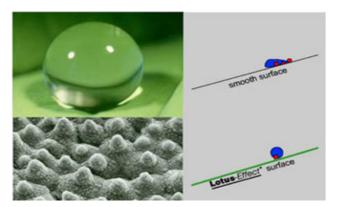
Figure 3: self-cleaning - lotus effect work mechanism and the different way of how the water droplet acts when touches a smoothe surface and surface with lotus effect
