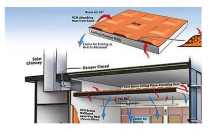
Figure 11: PCMs application in interior spaces in different parts walls and ceiling and how it changes material state (phase) according to the temperature and the day
