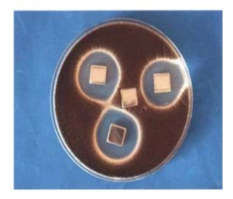
Figure 14: Fungicidal coatings on stainless steel plates reduce the formation of the mould aspergillus niger
