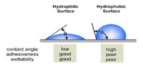
Figure 5: Easy to Clean on hydrophilic and hydrophobic surfaces and the difference of the adhesiveness between both surfaces
