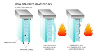
Figure 12: Fireproof Glass Panels Internal activation mechanism
