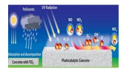
Figure 6: Air-purification coating on outdoor surfaces and activation process.
