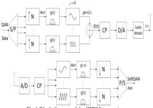
Fig.1 Block diagram of the GFDM transceiver
