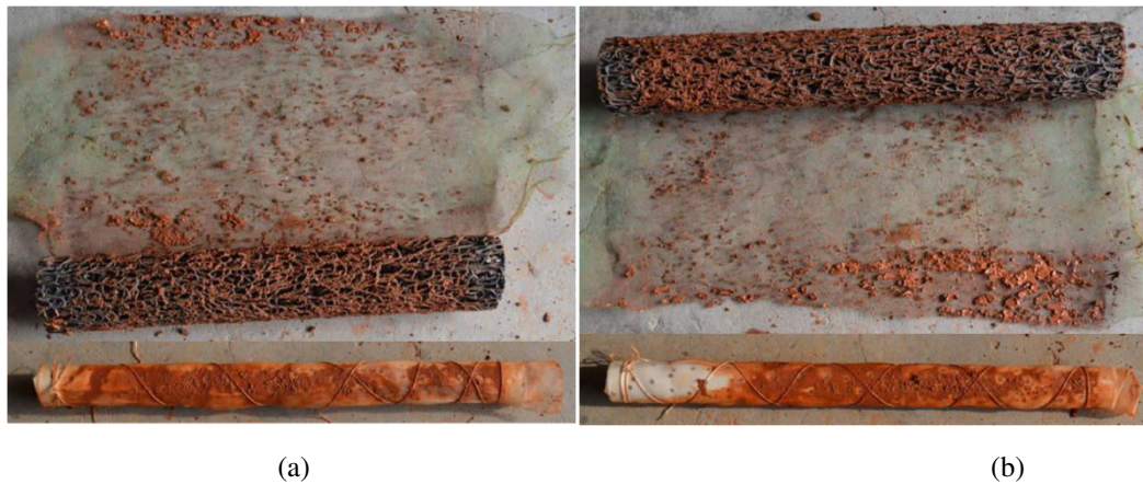
Fig. 8. B 2-1 Drainage pipe after the end of the experiment (a) B 2-2 Drainage pipe after the end of the experiment (b)
