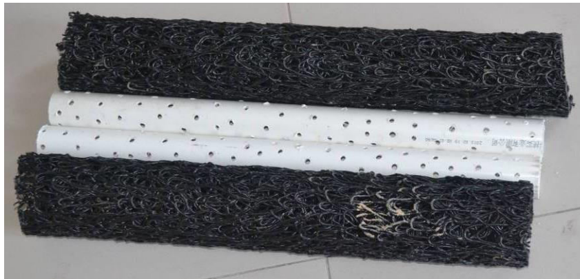
Fig. 2. Experimental Drainage Pipe
