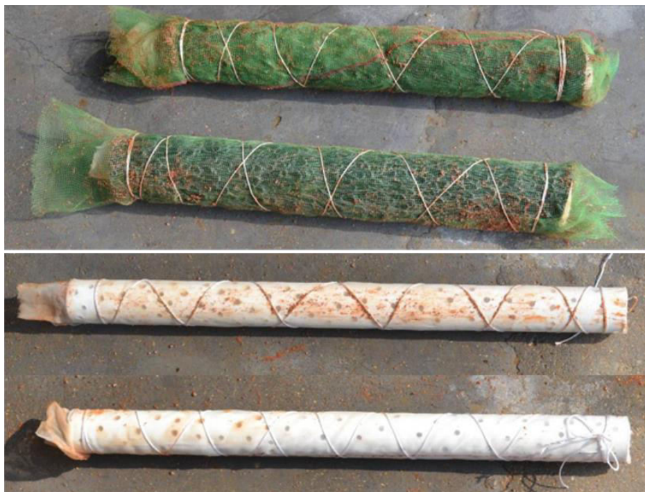
Fig. 6. B 1 Drainage pipe after the end of the experiment
