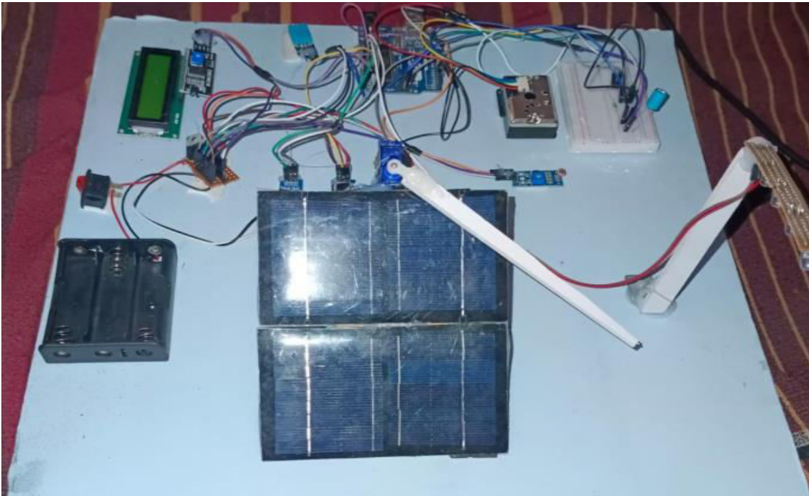
Fig 4.1 arduino based solar power system with automated cleaning wiper
