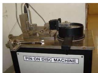
Figure 3.3: The pin on disc Wear test Apparatus.
