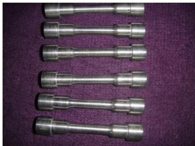
Fig.3.2: Tension test specimens
