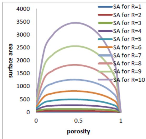
**Fig 5. SA (IN CM<sup>2</sup>) AGAINST POROSITY FOR VARIOUS 'R'**
