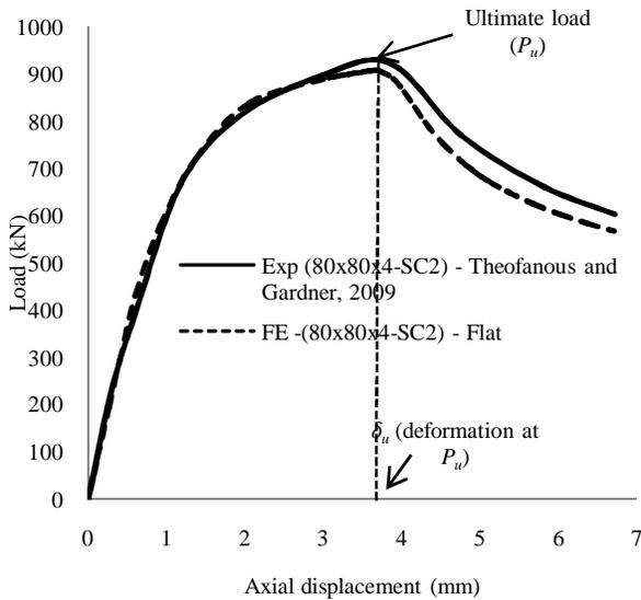
Fig. 4: Variation of load with axial displacement for square stub column (80x80x4-SC2).
