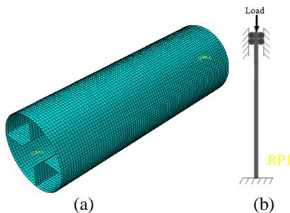
Fig 2: (a) FE mesh (b) boundary conditions for LDSS circular HC
