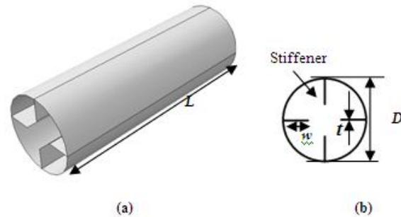
Fig 1: Schematic diagram of the LDSS hollow stub column/tube (a) isometric view, (b) sectional view ( $w$  = width of stiffener,  $D$  = diameter of column,  $L$  = length of column,  $t$  = thickness of stiffener)
