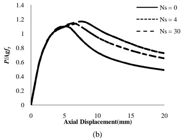
Fig. 5: (a) Variation of normalised load with axial displacement ( $w/D=0.1, t=3.75\text{mm}$ ) (b) Variation of load with axial displacement ( $w/D=0.1, t=3.75\text{mm}$ )
