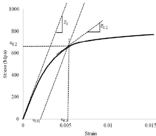
Fig 3: Compressive flat material properties (Theofanous and Gardner [19]).
