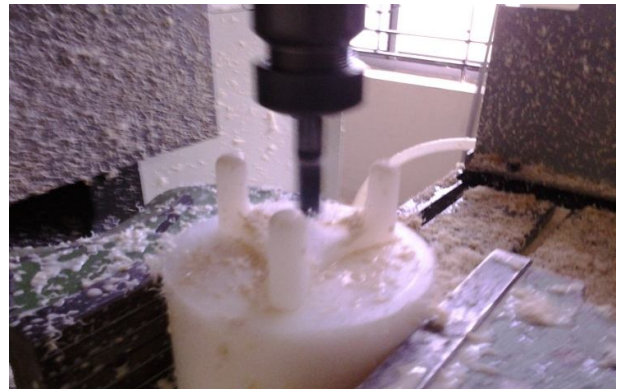
Figure 3 A view of the striker machining process
