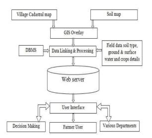
Fig1: Architecture for ALSI System
