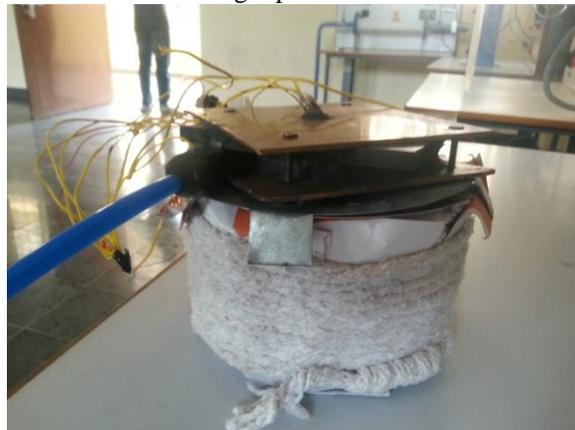
Figure 3: Final setup of the spiral flow heat exchanger
