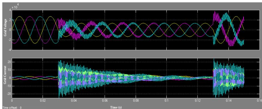
Fig.10 Grid Voltage & Current for PI Controller
