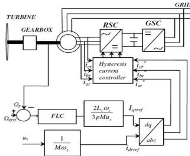
Fig.3 Block Diagram of the Rotor Side Converter Control
