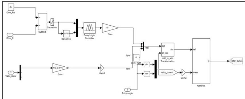
Fig.8 Rotor Side Converter Controller
