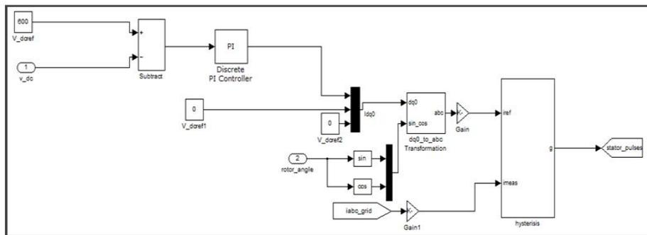
Fig.9 Grid Side Converter Controller
