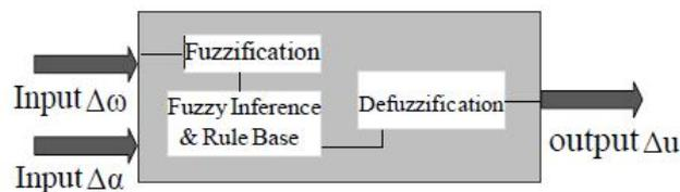
Fig.5 Block Diagram of the Fuzzy Controller
