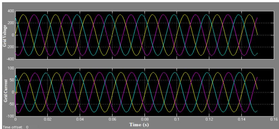
Fig.12 Grid Voltage and Current for Fuzzy Controller
