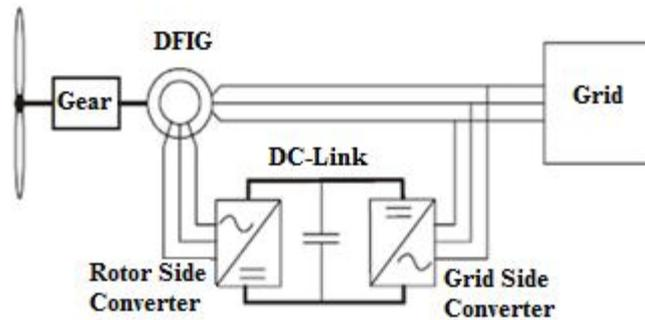
Fig.1 Scheme of the Wind System
