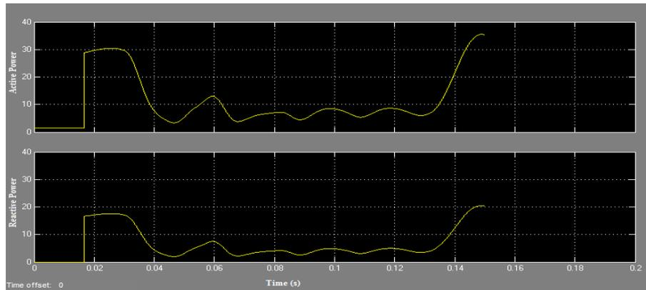
Fig.11 Active and Reactive Powers for PI Controller
