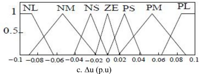
Fig.6 Triangular Membership Functions for Inputs and Output Fuzzy Sets of the Fuzzy Controllers
