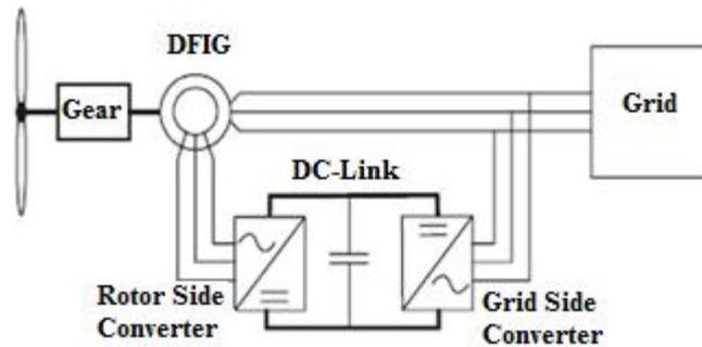
Fig.1 Scheme of the Wind System
