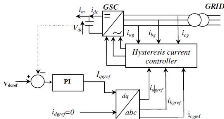
Fig.4 Block Diagram of the Grid Side Converter Control
