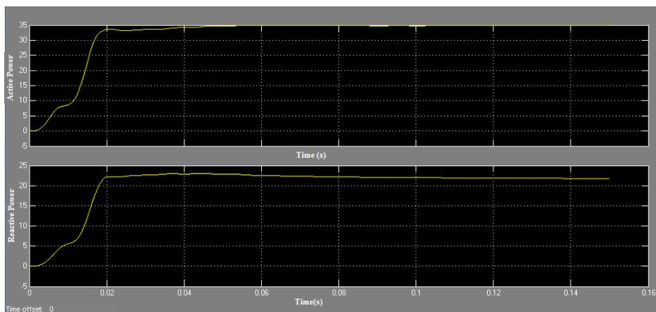
Fig.13 Active and Reactive Powers for Fuzzy Controller
