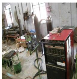
**Fig.3** Lincoln Electrical square wave TIG 355 Machine
