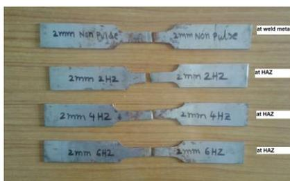
**Fig.4.** Tensile test specimens after test
