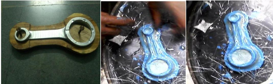
Fig 22: Mold Preparation
