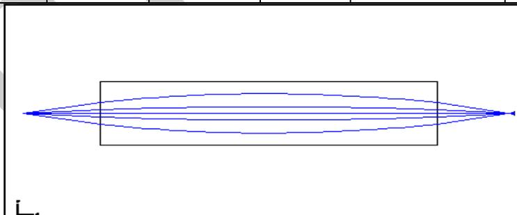
Fig (2) the structure of the gradient – index lens [11].
