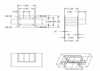
Fig.6 Diagrammatic Representation of the Electro Magnet using Pro E Software
