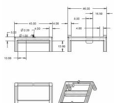
Fig.5 Diagrammatic Representation of the Frame using Pro E Software
