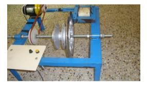
Fig 10. Front View of the Fabricated Brake System
