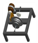
Fig.7 Assembled View of the Electro Magnetic Braking System using Pro E Software
