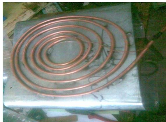
**Fig.3.** Ellipse Shaped Evaporator Coil
