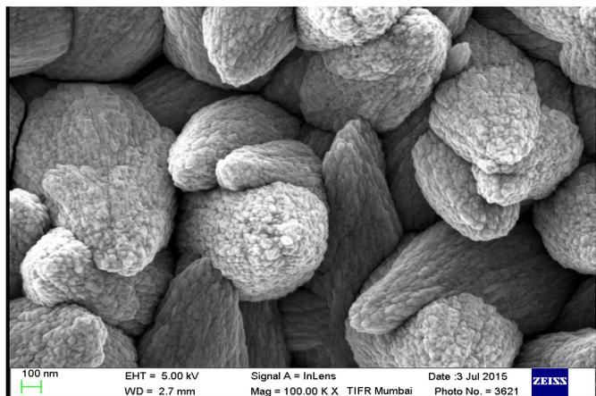
Fig. 2(b) : SEM images of ZnO thin film showing almond-like microcrystals
