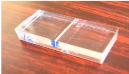
Fig. 1 Machined specimen in CO<sub>2</sub> laser machine by overlapping of lines
