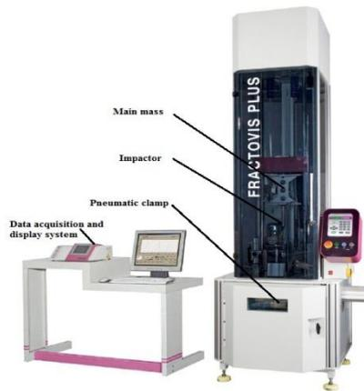
Fig.1 Impact testing facility
