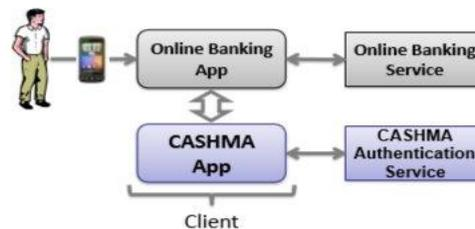
It is required that the user and the web service are en-rolled to the CASHMA authentication service. We assume that the user is using a smartphone where a CASHMA application is installed.
