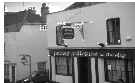
Fig.1 Original image used as input Fig.2 Output after passing through Gaussian filter with sigma=1 and Threshold=100 for Harris corner detector
