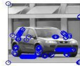
Fig.9 Corner detection using susan corner detector
