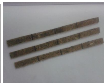
Fig 2.1.2: pattern of kenaf & coir/Epoxy composite specimen
