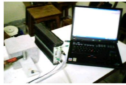
Fig2.4.1: Modal Hammer Fig2.4.2:Bruel & Kajer FFT Analyzer Fig2.4.3:Vibration testing of GFRP
