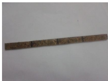
Fig 2.1.2: pattern of kenaf & coir/Epoxy composite specimen
