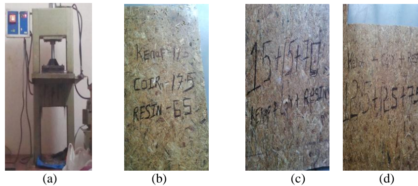
Fig. 1 (a) Compression Moulding Machine (b) Kenaf+coir+epoxy resin (17.5%+17.5%+65%) (c) Kenaf+coir+epoxy resin (15%+15%+70%) (d) Kenaf+coir+epoxy resin (12.5%+12.5%+75%)
