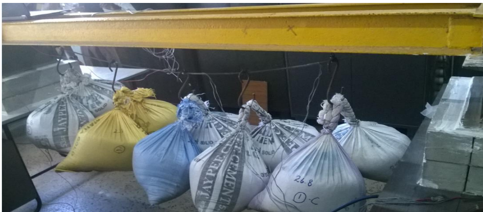
FIG:5 CABLE WITH APPLIED LOADS
