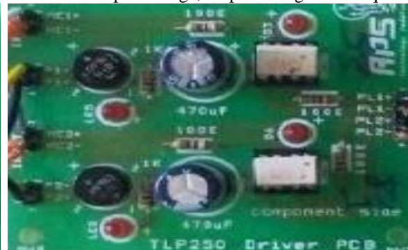
Fig 6.3 Two optocoupler circuit in a single PCB
