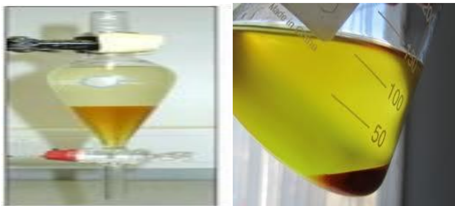
Fig 3. Separation of biodiesel from glycerol
