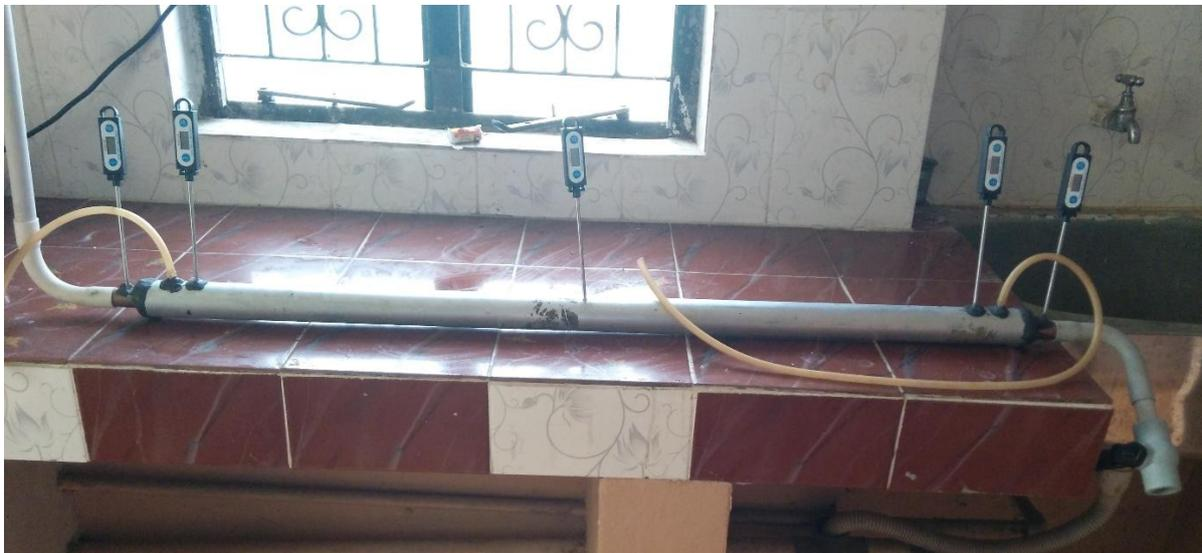
It consists of copper pipe inside the aluminum pipe with the annular space of 16 mm. both the ends of aluminum are sealed with thermo seal (m-seal), the aluminum pipe is bored with 5 holes. In which water proof digital thermometers are fitted in 3 holes to measure the inlet, outlet, flow temperatures.
