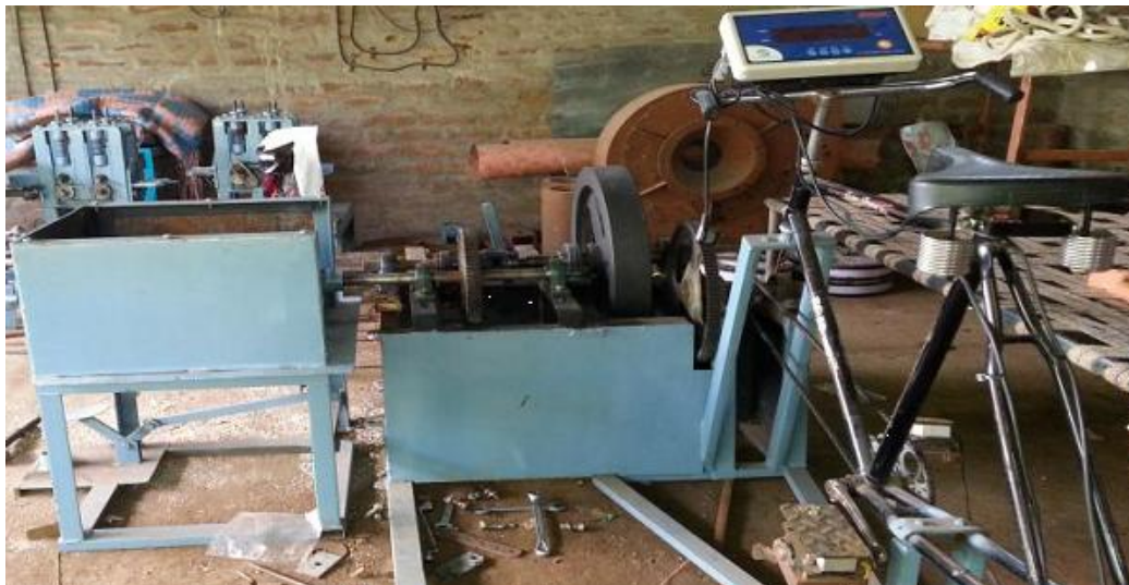
Figure 6: Fabricated set up for stirrup making machine
