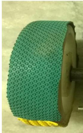
Figure 4 :- Nylon wheel with grips
