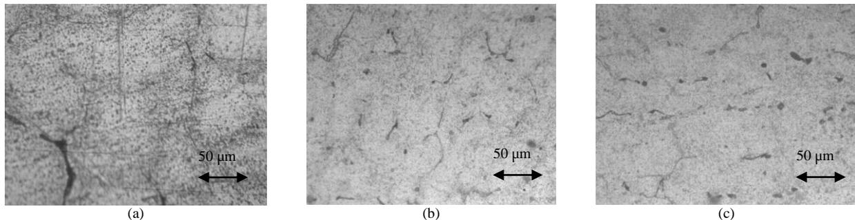
Fig. 1: Optical micrographs of Al 6061 alloy and its hybrid composites (a) Al 6061 alloy, (b) Al 6061-5wt%SiC/1wt%Gr Composite and (c) Al 6061-10wt%SiC/1wt%Gr Composite
