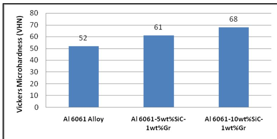
Fig. 2: Variation of microhardness with increase in reinforcement
