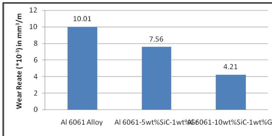
Fig.3: Effect of reinforcement on volumetric wear rate of Al 6061 alloy
