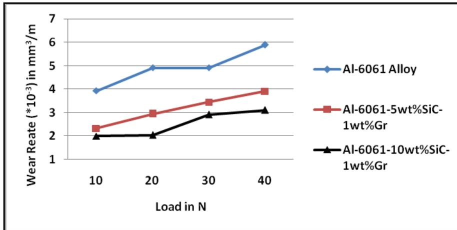
Fig.4: Effect of load on volumetric wear rate of Al 6061 alloy and its hybrid composites
