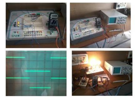
This images consists of zero crossing detector circuit connection and its output. The output is seen by using CRO. The CRO monitor shows two waveforms the first wave form is voltage waveform and the second one is current waveform.
