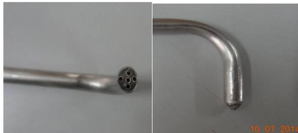
Fig 1. Fabricated five hole probe with 90° bend
