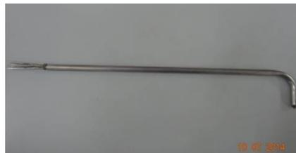
Fig. Fabricated Five Hole Probe
