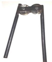
Fig 2. Tube bender mechanism
