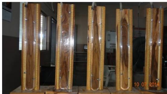
Fig 3. U tube manometer set-up
