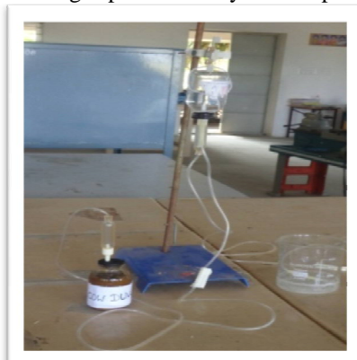
Fig. (2) Analysis Of Gas Production By Water Displacement Method.
