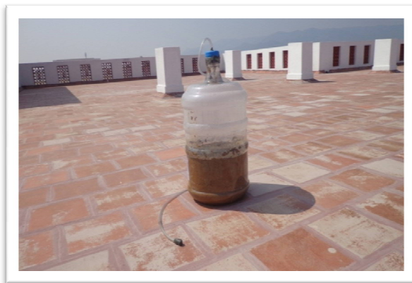
Fig. (6) Waste kept for degradation in the sealed reactor.
