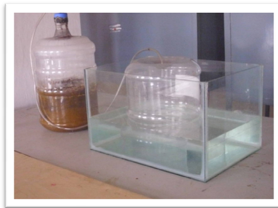
Fig. (8) Reactor Set up for analysing the gas production.
