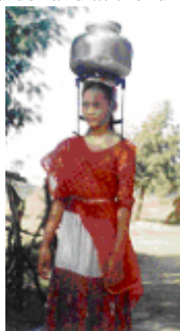
Fig. 7 : Panihari, a load reducing device developed by Khimjibhai Kanadia
