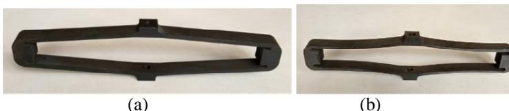
**Figure 9 Fabricated Flexural Amplifier design-1 and design-2**
