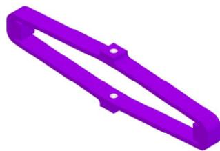
**Figure 3(a) Flexural Amplifier design-1**
