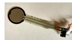
**Figure 10 Force sensing Resistor(FSR)**
