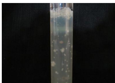
Figure 1(a): Growing crystals within the test tube Figure 1(b): Grown crystals of shiny white colour having spherulitic morphology
