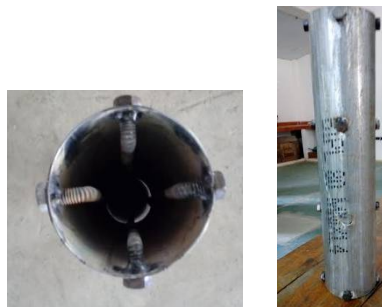
Fig.6. Steel tube with shear connectors before filling concrete
