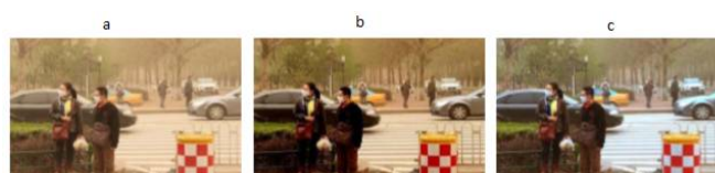
Fig 5.2 Results for input images with color distortion(a. sand storm image with colour distortion ; b.recovered image produced by previous method ; c.recovered image by our method )
