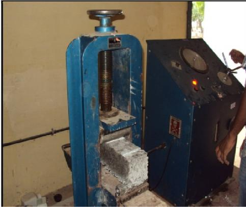
**Fig.5 Flexural Test on Pervious Concrete Prism**
