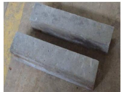
Fig. 4.15 Normal Concrete Prisms
