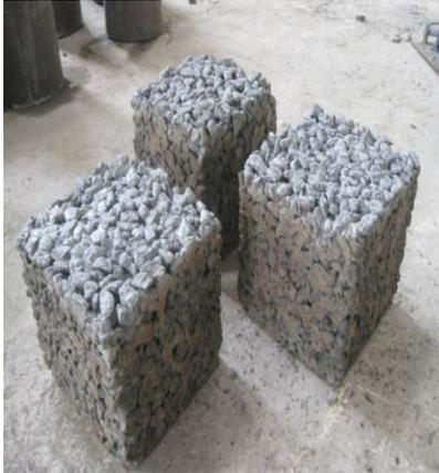
Fig.9 Pervious Concrete
