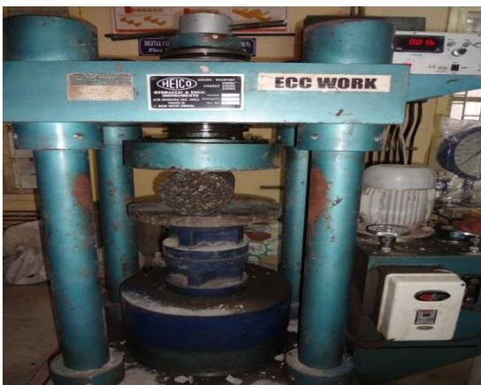
**Fig. 3** Split Tensile Test on Pervious Concrete Cylinders
