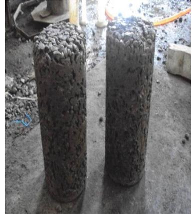
Fig.11 Pervious Concrete Cylinders
