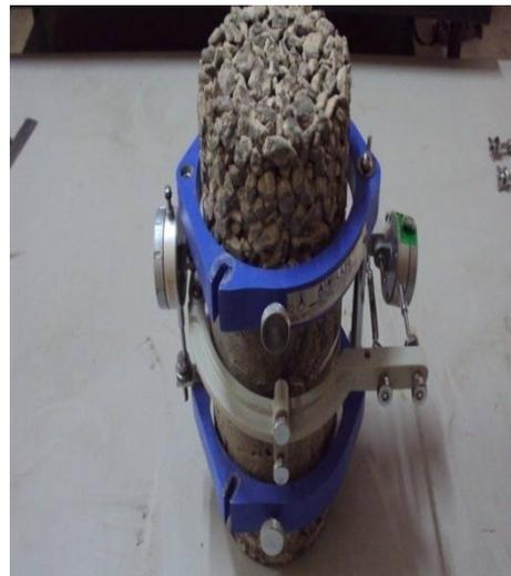
**Figure8 Poisson's Ratio Test Arrangement**
