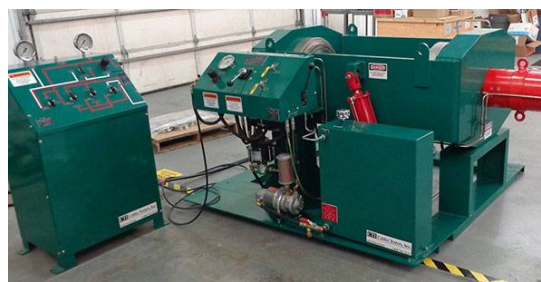
Fig 16 Test rig of check valve
