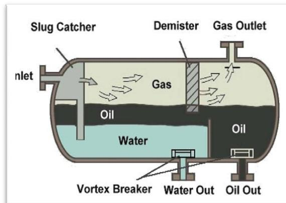
Fig.1. Separation process flow in horizontal gravity Separator
